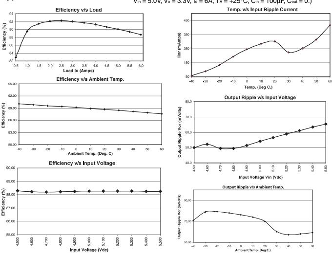
NOTE: The ambient temperature is as measured at approx. 1/4" away on the back side of the unit, with the probe end at approx. center (vertical & horizontal). For thermal performance, the unit was mounted on a 4"x4" PCB (with ground plane) & enclosed in a box so that it operates in a controlled environment.
